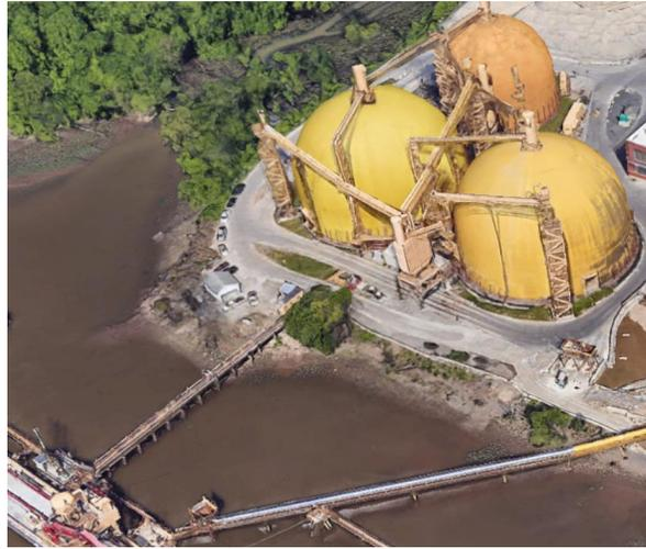
Located on the banks of the Delaware River, the Silvi Cement Terminal is the world's largest distribution center for concrete powder. The concrete powder is stored in large, pressurized domes.
